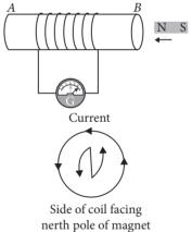
(b) Moved quickly away from coil: A current is induced in clockwise direction in the coil with respect to the side facing the north pole of the magnet and the needle of the galvanometer will deflect in opposite direction from case (a).
